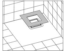
**NOTICE!** The Plancofix must be weighted down to keep it in position during application of the screed.
