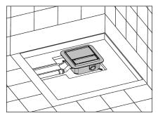
Conduits must be created for the pressure pipe and electricity supply cable, 1" FPT pressure pipe outlet, 3/4" cable conduit.
