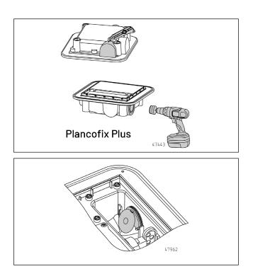
The Plancofix can also be installed in front of, or adjacent to, the shower. In this case, the shower is connected to one of the inlet connections at the side with a DN50 pipe socket.
