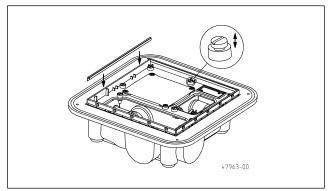
Both of the stainless steel cover elements (a) can also be completely tiled over (b). To do so, just turn the larger element over, and use the smaller element without a drain.
