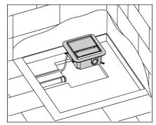
The Plancofix is recessed entirely into the floor. The unit can be accessed for maintenance through the top cover (tiled or stainless steel finish).
